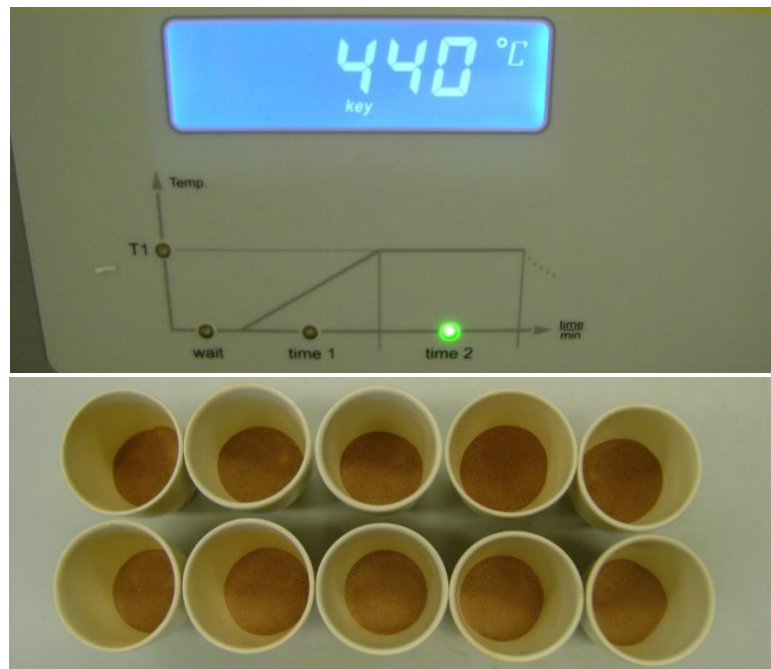
Fig. 3. Burning temperature 440°C in muffle furnace L 9/11/B180 (upper) and ten specimens (TestNo1 to TestNo10) of soil sample U1 taken from Ujsoly after burning (lower).
